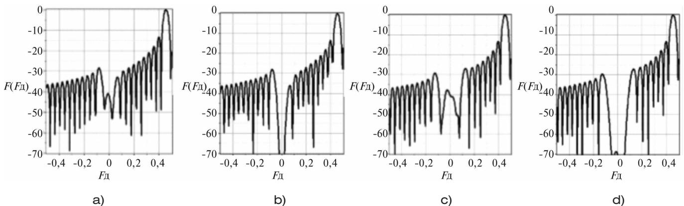
Figure 3. AFC of MTI RLS1L122 for rejection zone with five poor frequency responses for data accuracy: a – 14 digits after decimal point and b – 16 digits after decimal point; with seven poor frequency responses for data accuracy: c) – 24 and d) – 26 digits after decimal point
