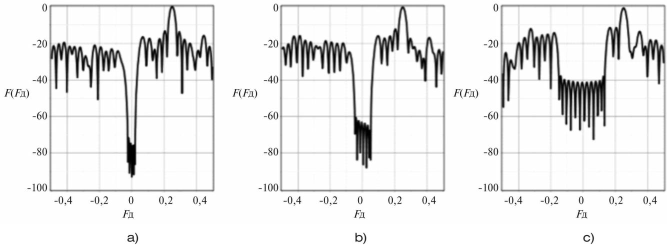
Figure 2. AFC of frequency filters with rejection zone width  $\pm 0.025 \Delta F$  (a),  $\pm 0.05 \Delta F$  (b),  $0.15 \Delta F$  (c), received using the method of limited optimization for the batch of 32 impulses
