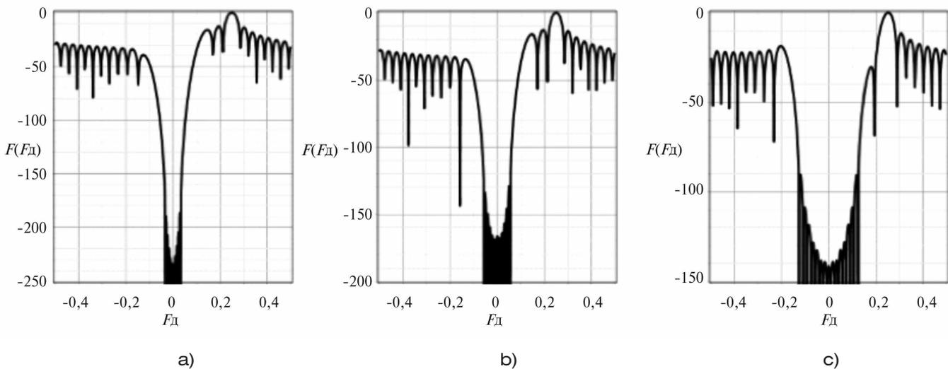
Figure 4. AFC of frequency filters with rejection zone width  $\pm 0.025 \Delta F$  (a),  $\pm 0.05 \Delta F$  (b),  $0.15 \Delta F$  (c), for the batch of 32 impulses, received by deterministic compensation method
