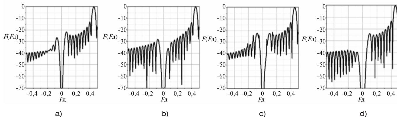
Figure 5. AFC of deterministic MTI for the rejection zone with 5 poor frequency responses (a, b) and 7 poor frequency responses (c, d) with data accuracy 10 and 12 digits after decimal point.
