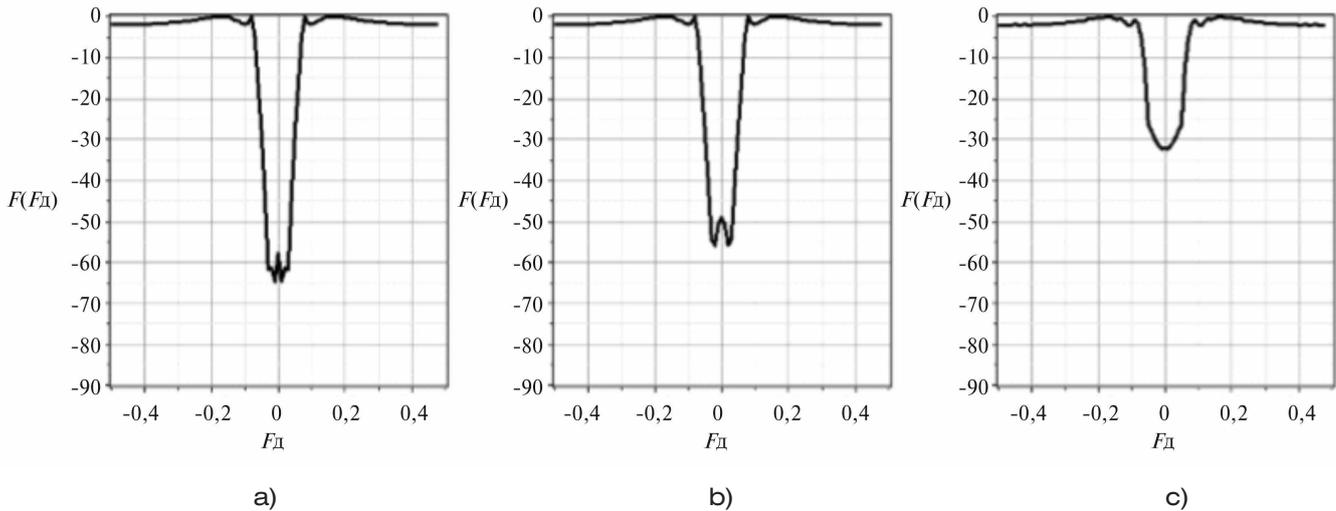
Figure 1. The elliptical quartic filter AFC dependence on the number of input impulses when  $N_{\text{in}} = 200$  (a), 100 (b) and 32 (c)
