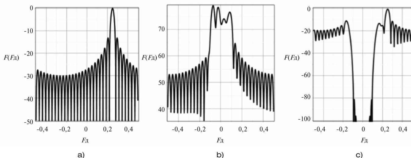
Figure 6. Bandwidth of useful signal with frequency  $0.25 \Delta F$  (a), the mixture of signals with interference (b) and useful signal after compensating passive interference at the passive interference bandwidth equal to  $\pm 0.1 \Delta F$  and signal/interference ratio  $-80$  db (c)
