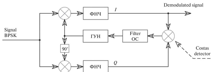
Figure 1. Costas circuit for demodulation of phase-shift keyed signals:  $I$  – common-mode signal;  $Q$  – quadrature signal; ФНЧ – low-pass filter; OC – feedback;  $90^\circ$  – phase-shifting unit; ГУН – voltage-controlled oscillator
