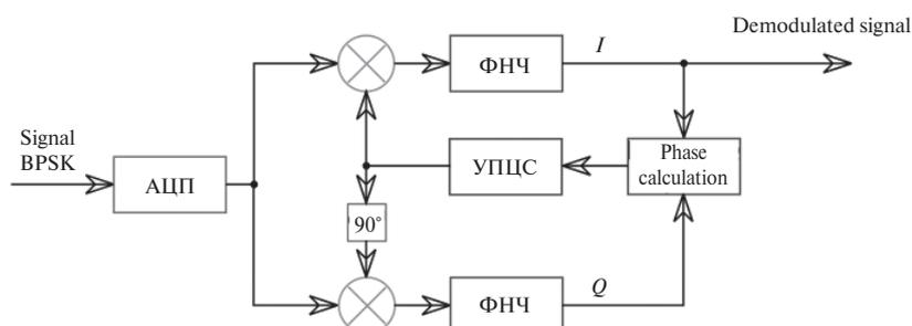
Figure 2. Functional diagram of the demodulation algorithm: АЦП – analog-to-digital converter
