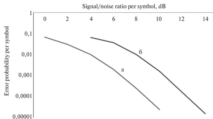
Figure 4. Dependence of the probability of incorrect  $P_B$  symbol reception on the signal-to-noise ratio resulting from: a – approximate calculation of the Gauss error integral; b – experimental studies
