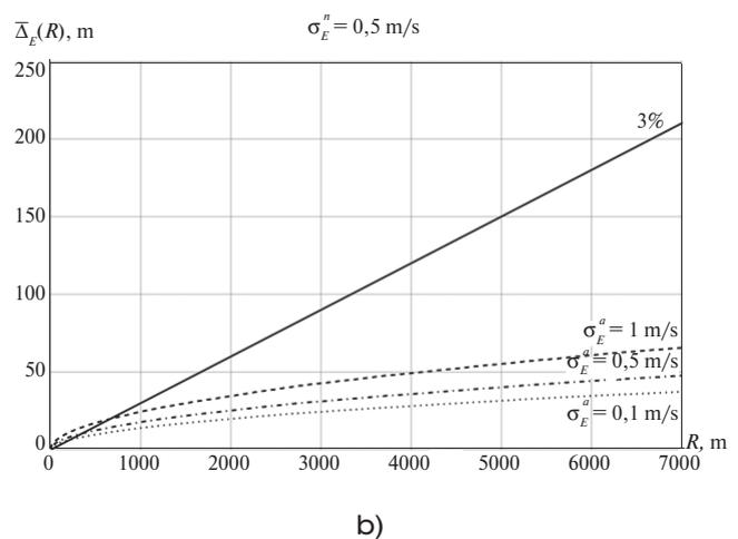
Figure 6. Dependence of the mean square positioning error  $\bar{\Delta}_E(R)$  on the travelled distance: a) for different  $\sigma_E^n$ ; b) with different  $\sigma_E^a$
