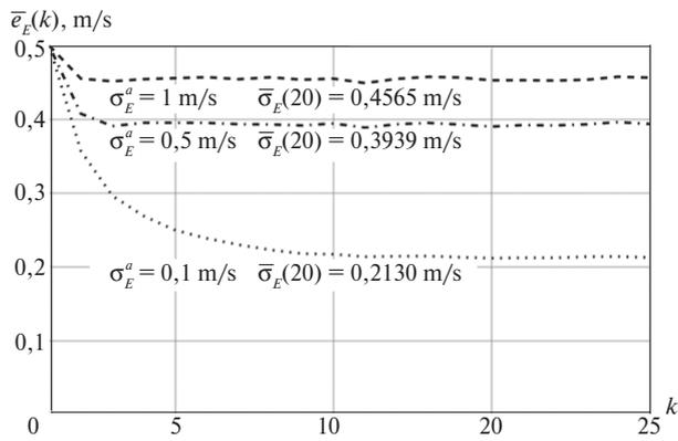
Figure 4. Plots of standard deviation in average sample  $\bar{\sigma}_E(k)$
