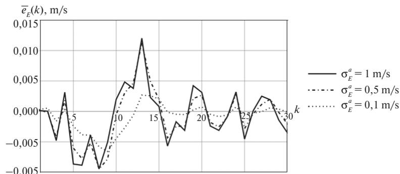
Figure 3. Expected value for the error in the eastern channel in average sample
