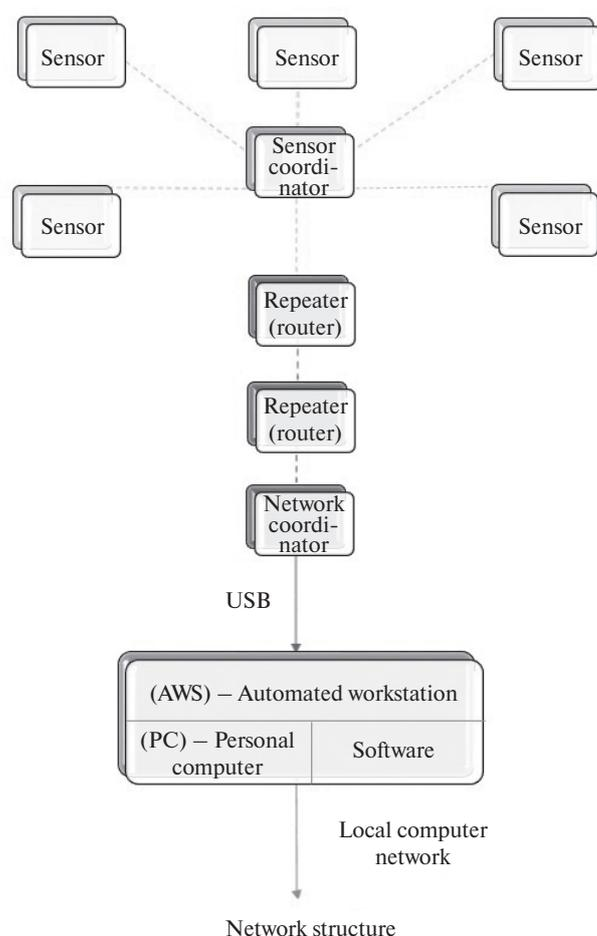
Figure 2. The architecture of the wireless data transmission network from the underground observation station to the operator's computer
