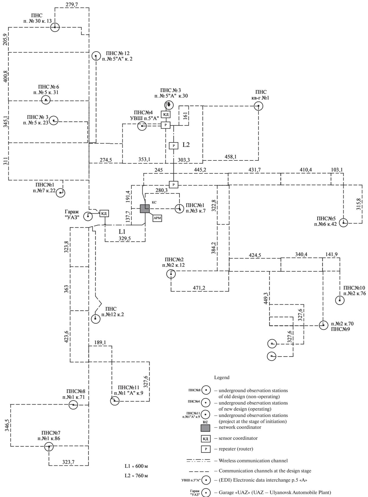
Figure 1. The architecture of wireless data transmission network from the underground observation station to the operator's computer.
